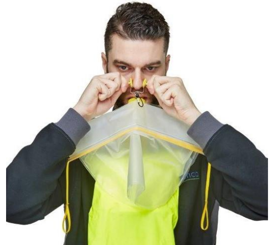
8. Adjust the neck strap, fit nose clip and exhale into the mouthpiece
