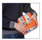
I. Open the yellow upper latch lever to remove the lid of the case. Discard the lid.
